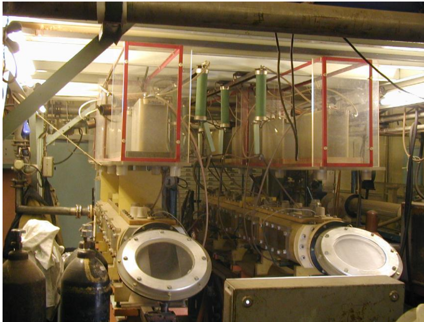
Fig. 2 – Laser cuvettes with Brewster windows of NaCl single crystals having a diameter of 300 mm
