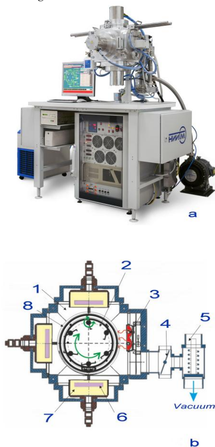
Fig. 1 – Main view (a) and schematic configuration (b) of “MVU TM-Magna 3M”. 1 – Working chamber, 2 – Planetary substrate holder, 3 – Ion-beam cleaning electrode, 4 – Throttle shutter, 5 – Commutator, 6 – Target, 7 – Magnetron, 8 – Cylindrical shutter
