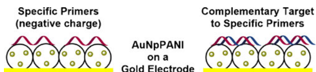
Fig. 12 Schematic representation the AuNpPANI on a gold electrode biosensor assembling (adapted from [77])
