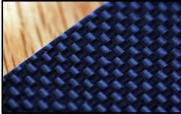
Figure 2.5: Example of carbon fiber reinforced plastic (Strong, 2008).
