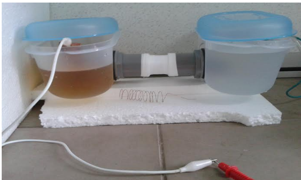
Figure 1.3: The setup for the bio battery using urine
