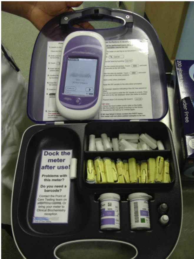
Fig. 2. A blood glucose meter with accompanying case and paraphernalia, i.e. swabs, lances, vials containing test strips and two plastics bottles containing fluid for quality control procedures.
