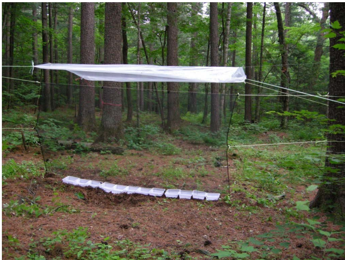
Figure 15 Window trap using black silk mesh of 1.5m x 3m with a plastic roof
