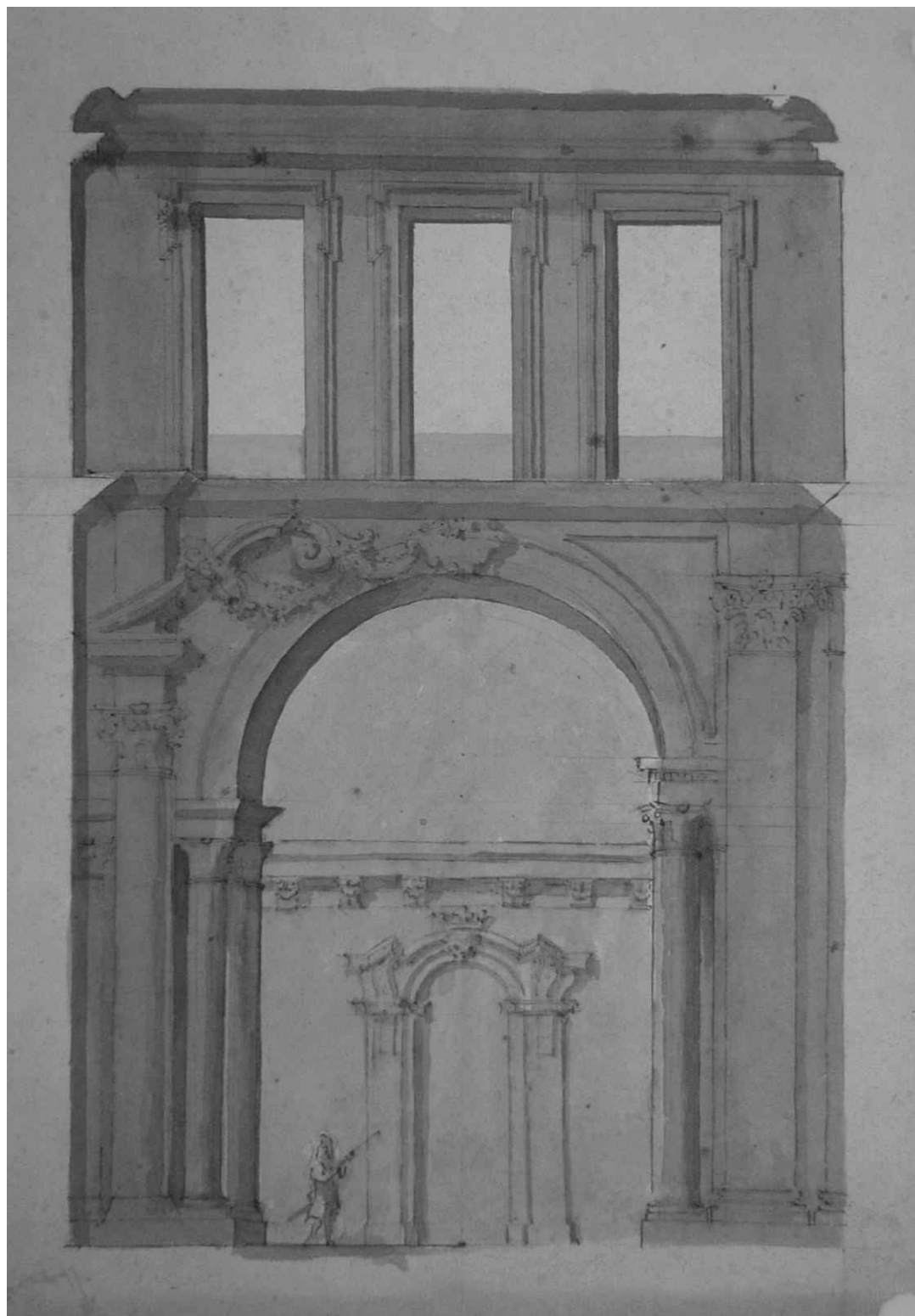
Fig. 70 Nicholas Hawksmoor, Transverse Section of the Great Hall, Blenheim Palace , showing proposed treatments for the southern wall, mid-1707, Minet Public Library, Lambeth, London
