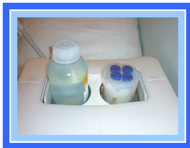
Figure 3.22- Phantom setup for sequence testing
