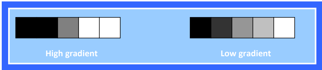
Figure 2.16- Pictorial depiction of high and low gradient in an image when considering the three central pixel grey levels
