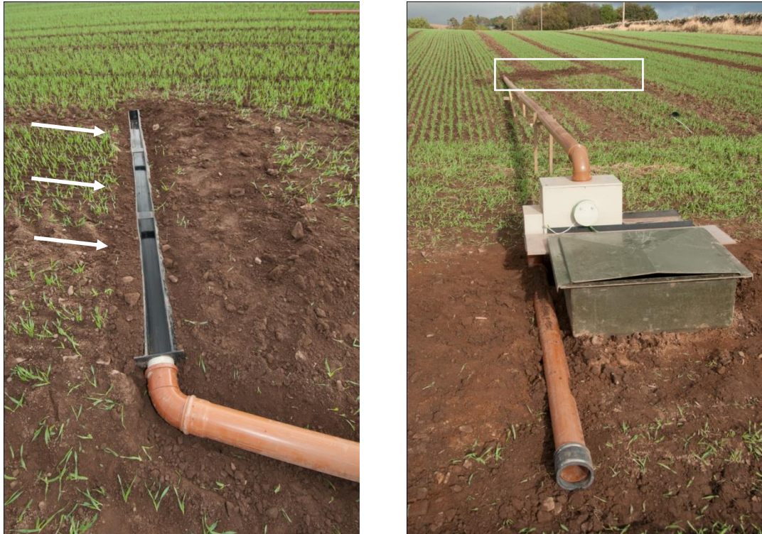
Figure 2.4 - Runoff material from the tramlines (shown by white arrows) was collected in the Gerlach Trough (left and highlighted in right) and piped into the tipping bucket situated above the storage tank (right). Sub-samples were stored in the tank and excess material discharged down the waste pipe.
