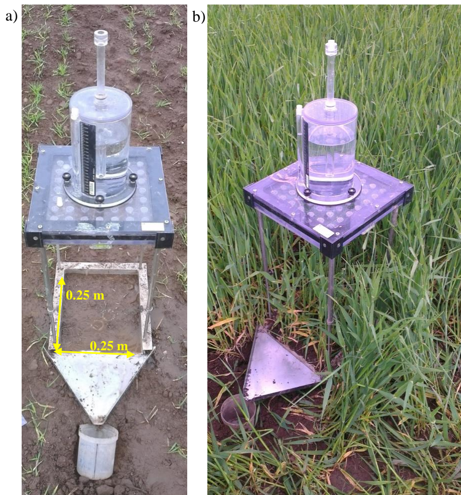
Figure 4.3 - Kamphorst (1987) rainfall simulator being used in the field. On a tramline (a) the rainfall simulator demonstrates rain splash and runoff. The difficulties of use in tall vegetation are demonstrated in (b).
