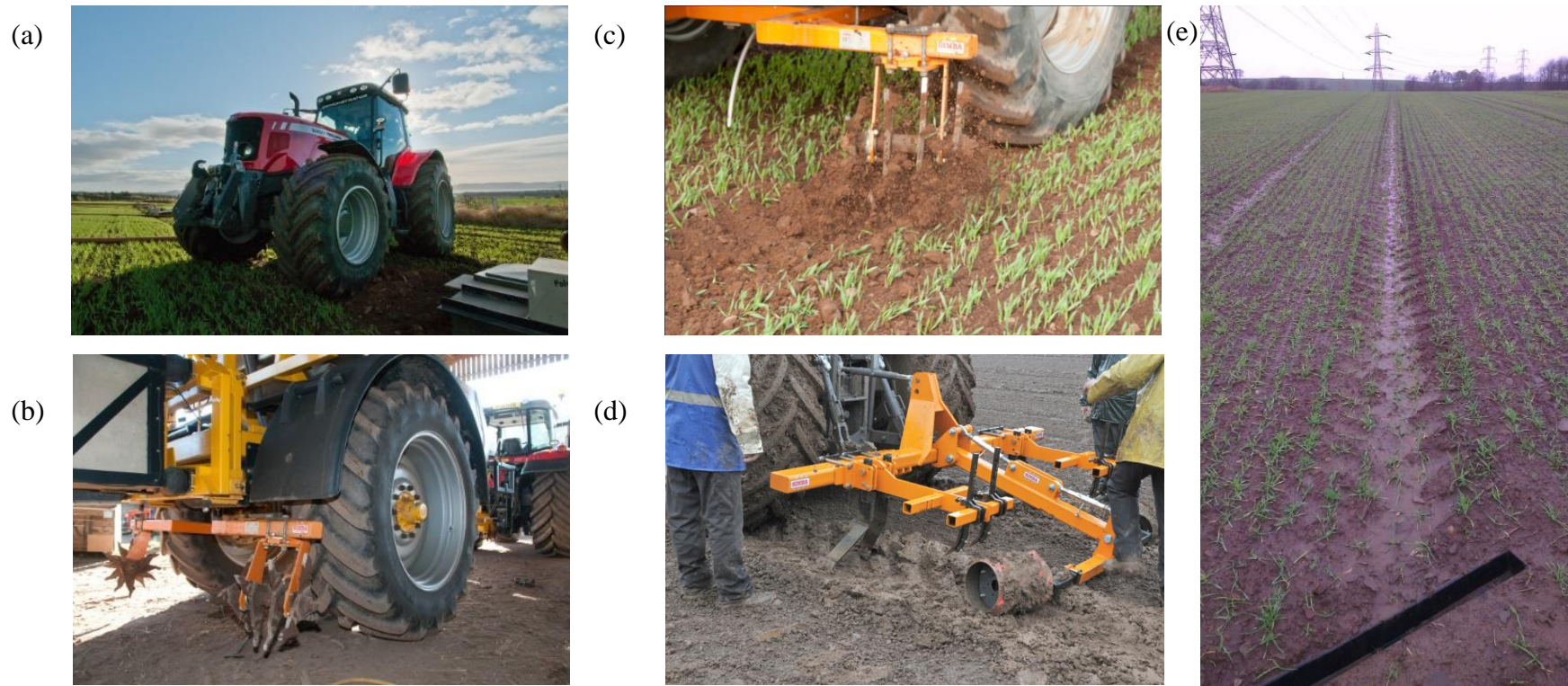
Figure 2.1- Tramline management techniques showing the (a) regular tyre, (b) low pressure tyre, (c) spiked cultivator breaking up the tramline surface, (d) the roller creating a convex channel shape; and (e) typical tyres tramline sown with Hordeum vulgare during winter in 2012/13.
