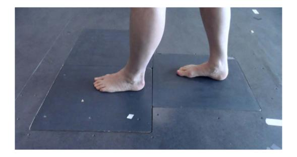
Figure 2.3 Kistler<sup>®</sup> force plates sunk into a permanent walkway
