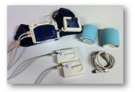
Figure 2.4 F Scan<sup>®</sup> system with insoles which can be cut to size
