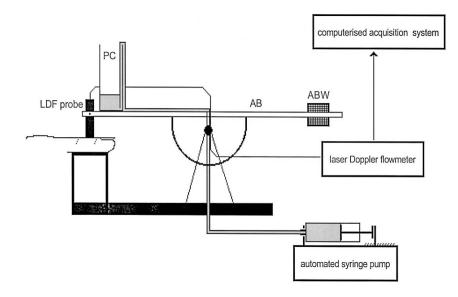
Figure 2.12 The mechanical device developed by Fromy *et al.* (2000). The device was used to apply a progressive calibrated pressure to a local area of skin and simultaneously measure cutaneous blood flow with a laser Doppler probe at the same site. PC: plastic container; AB: aluminium bar; ABW: adjustable balance weight (adapted from Fromy *et al.*(2000).
