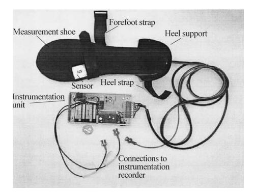
Figure 2.13 Measurement shoe and waist mounted instrumentation unit, with the sensor situated under first metatarsal head (adapted from Cobb & Claremont 2001).
