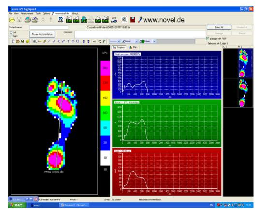
Figure 4.1 Emed-x/E pressure analysis system with peak plantar pressures displayed in kPa during walking
