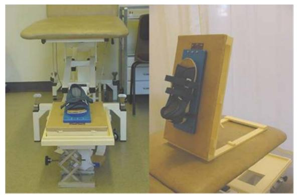
Figure 2.14 The device in a semi-weightbearing position (adapted from Santos et al. 2003)
