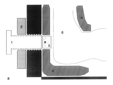
Figure 2.11 The experimental set-up: 1, spindle mechanism; 2, load cell; 3, board at the end of the bed; 4, shoe; 5, LDF probe with the laser source; and two photodiodes detecting the reflected light; 6, foot (adapted from Meinders *et al.* 1996).
