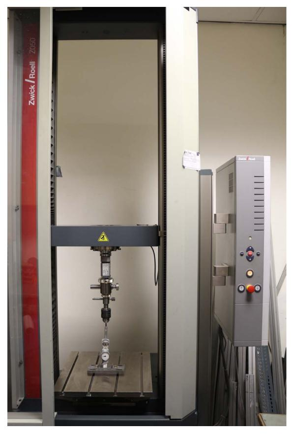
Figure 3.6 Universal testing machine (Zwick Roell) with the pressure delivery device in situ
