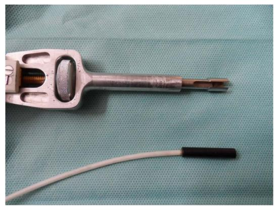
Figure 3.1 The pressure delivery system displaying the housing 'cuff' and the LDF probe
