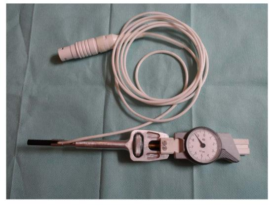
Figure 3.3 The pressure delivery system with DP2 probe attached allowing freedom for the optic fibres to function unimpeded
