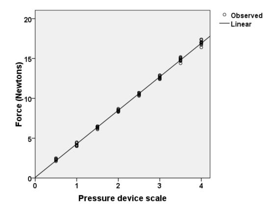
Figure 3.7 Linear relationship of the pressure device scale and applied forces
