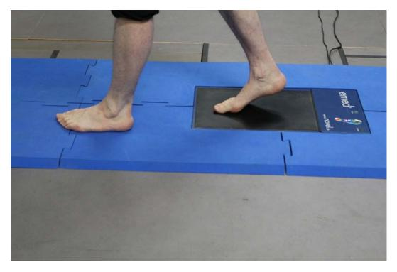
Figure 2.2  $\operatorname{Emed}^{\circledast}$  platform system in conjunction with portable walkway
