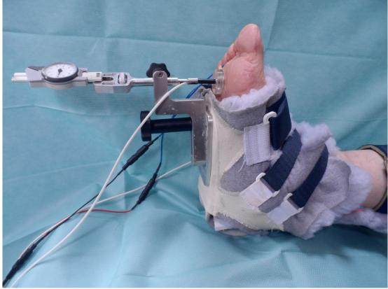
Figure 4.5 The pressure delivery system held in position via the adapted boot with the iontophoresis chamber housing the laser Doppler probe and the solutions with the vasodilators
