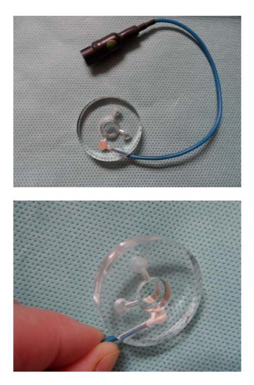
Figure 3.9 The chosen MIC1-Ion1 chamber. Dimensions of the elements of the chamber are a central aperture of 6.1mm and three connecting apertures each 4mm in diameter connected by a 2mm drill which allows flow of solution and top up when required.
