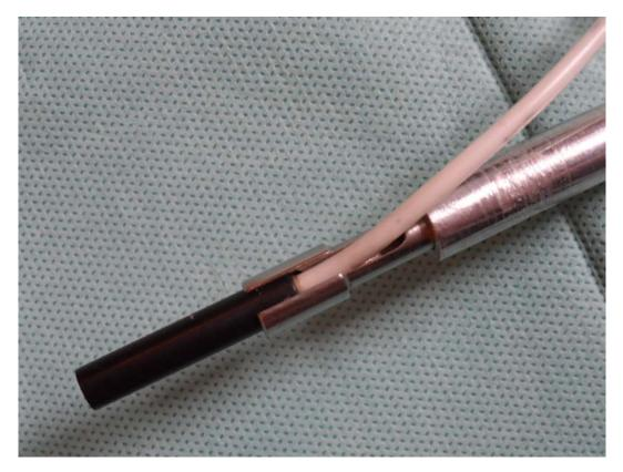
Figure 3.2 DP2 probe held within the base of the pressure delivery system
