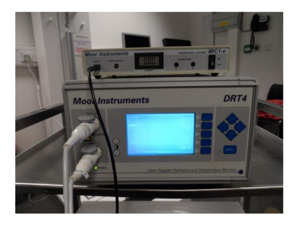
Figure 2.9 Laser Doppler flowmeter utilised in conjunction with an iontophoresis controller
