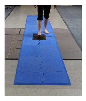
Figure 4.2 Emed-x/E pressure analysis system set into the portable walkway
