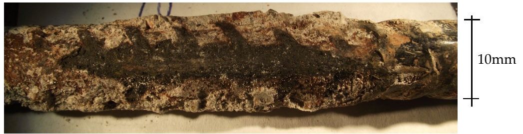
FIGURE 5.16 BLACK CORROSION PRODUCT (NEGLIGIBLE OXYGEN)
