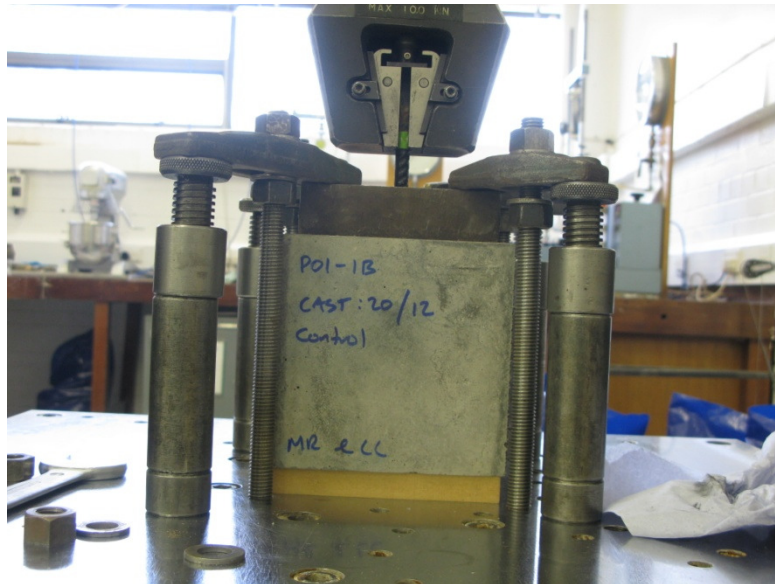
FIGURE 3.30 PULL-OUT TEST EXPERIMENTAL SETUP
