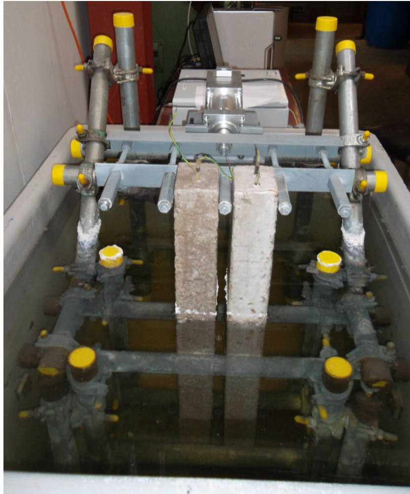
FIGURE 3.25 SETUP OF DYNAMIC BEAM LOADING IN SUBMERGED ENVIRONMENT
