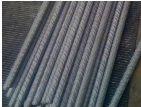
a) grit blasted reinforcing bar
