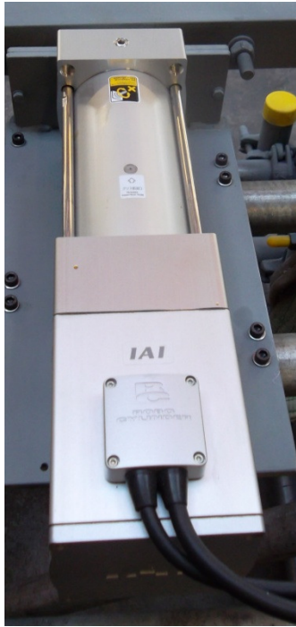
FIGURE 3.21 ROBOCYLINDER RCP2 ACTUATOR
