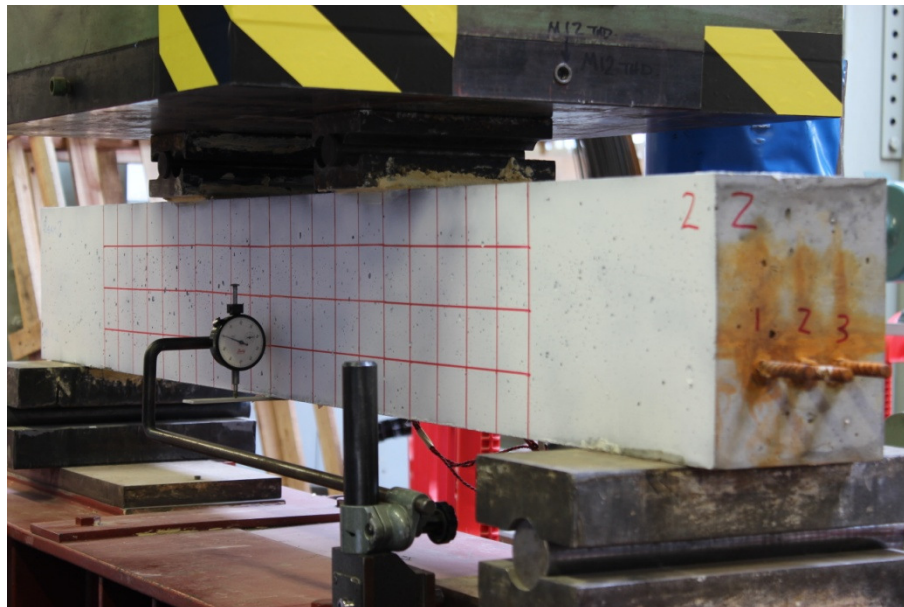
FIGURE 3.31 FOUR-POINT BENDING TESTING WITH DEFLECTION AND STRAIN MEASUREMENTS
