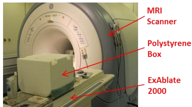
Figure 4.11- UF sonoporation arrangement covered by a polystyrene box
