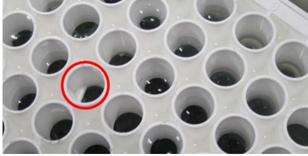
Figure 4.13- Deformation in a single well due to FUS (marked in red)
