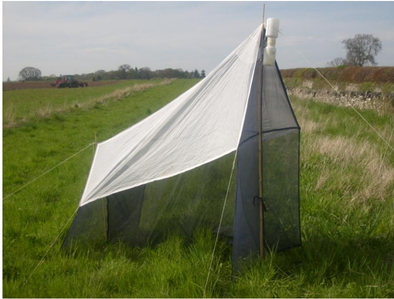
Plate 2.1: Malaise trap in side-view identical to those used in the study.
