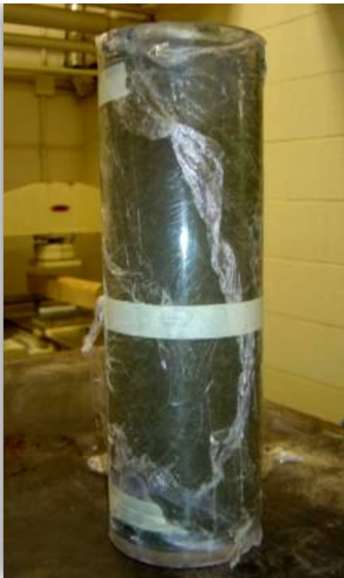
Figure 3.13: Foamed concrete freshly poured into cylinder
