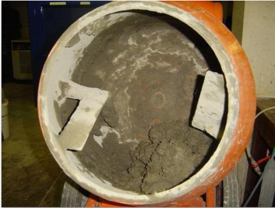
Figure 4.6: Base mix in rotary mixer
