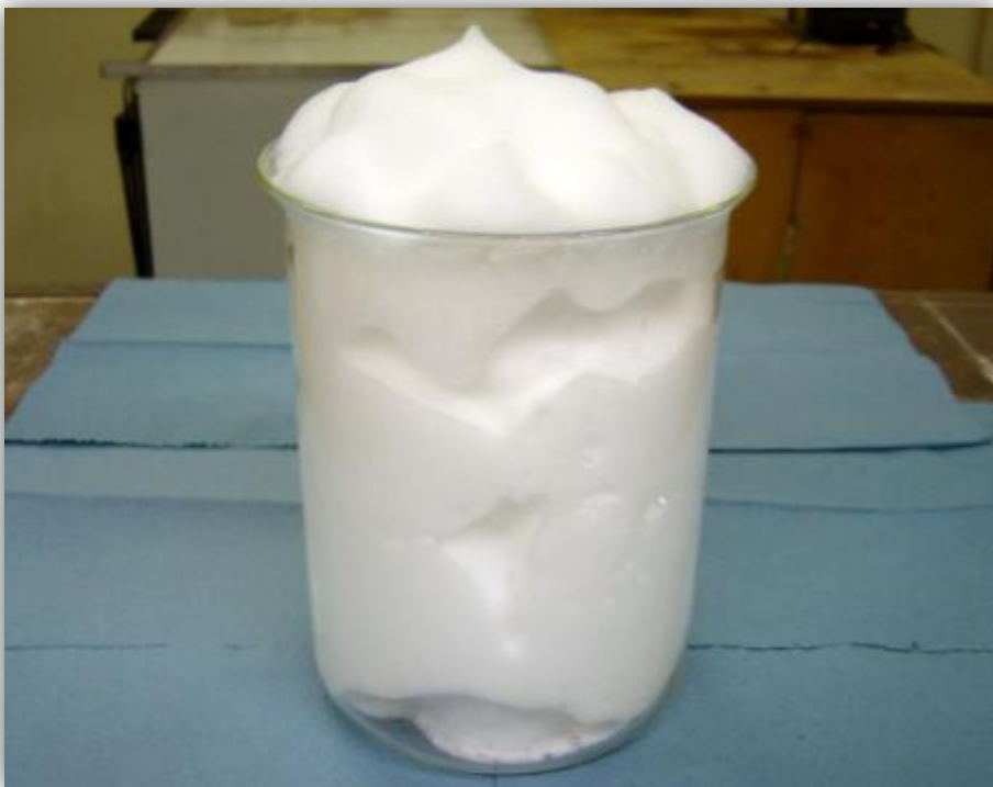
Figure 3.9: Foam in a jar for density check
