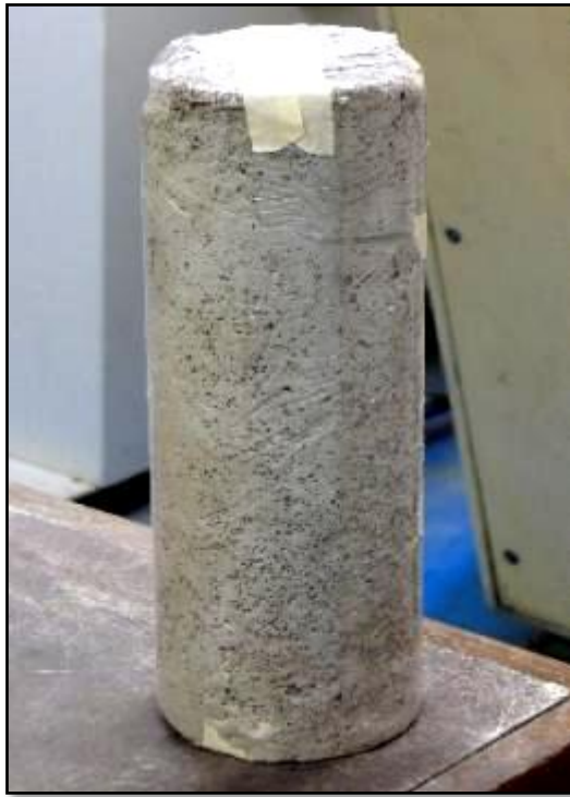
Figure 6.2: Foamed concrete specimen wrapped in 'cling' film
