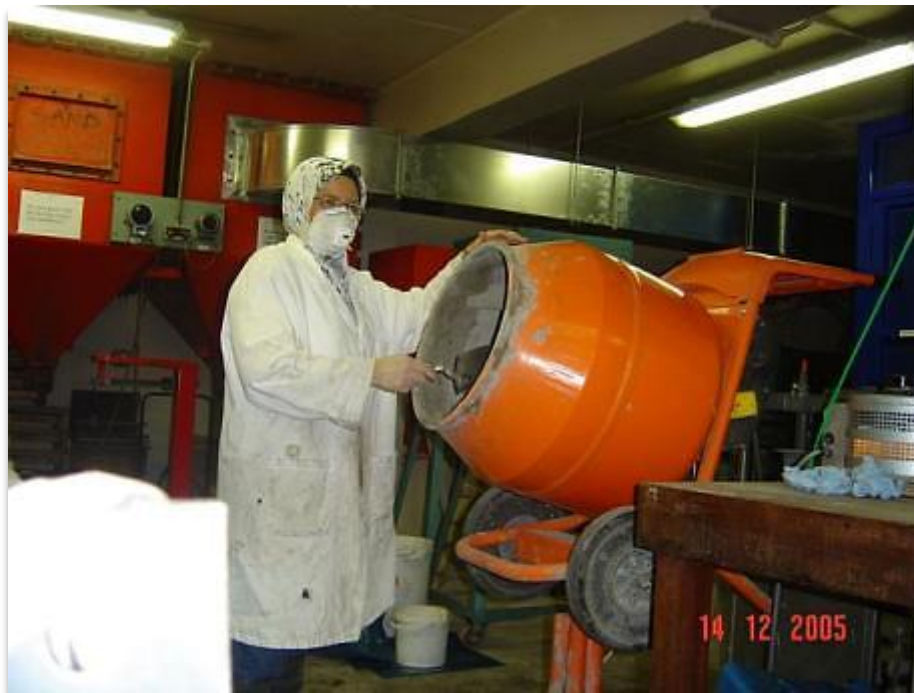
Figure 4.5: Foamed concrete mixed in a standard inclined rotating mixer
