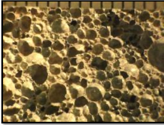
Figure 6.21: Density 600 kg/m 3 at w/c ratio 0.50 without wetting agent
