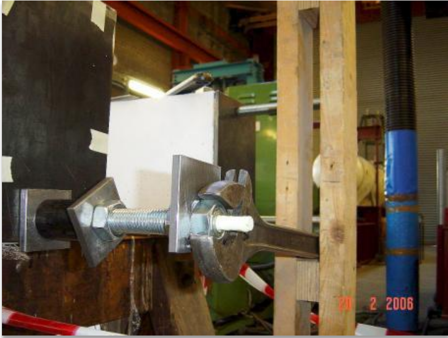
Figure 4.14: Close-up detail of tensioned end
