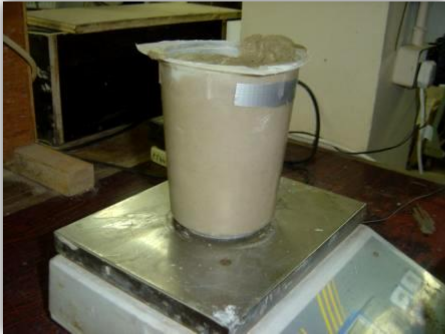
Figure 3.12: Density check for foamed concrete
