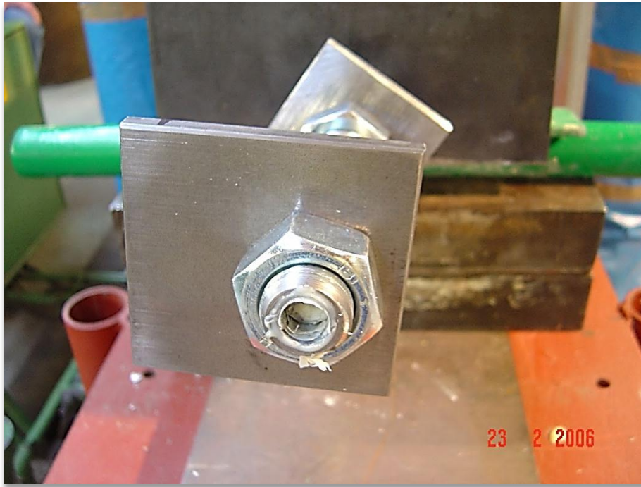
Figure 4.18: The reinforcement creep and did not sustain the added tension in the beam
