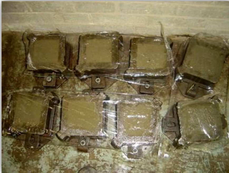
Figure 3.15: Cubes covered with 'cling film' and placed at room temperature 20 \pm 2^\circ\text{C} before demoulding
