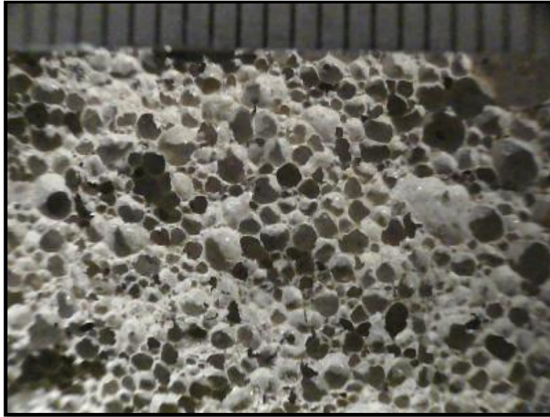
Figure 6.17: Density 600 kg/m 3 at 0.50 w/c ratio using protein surfactant
