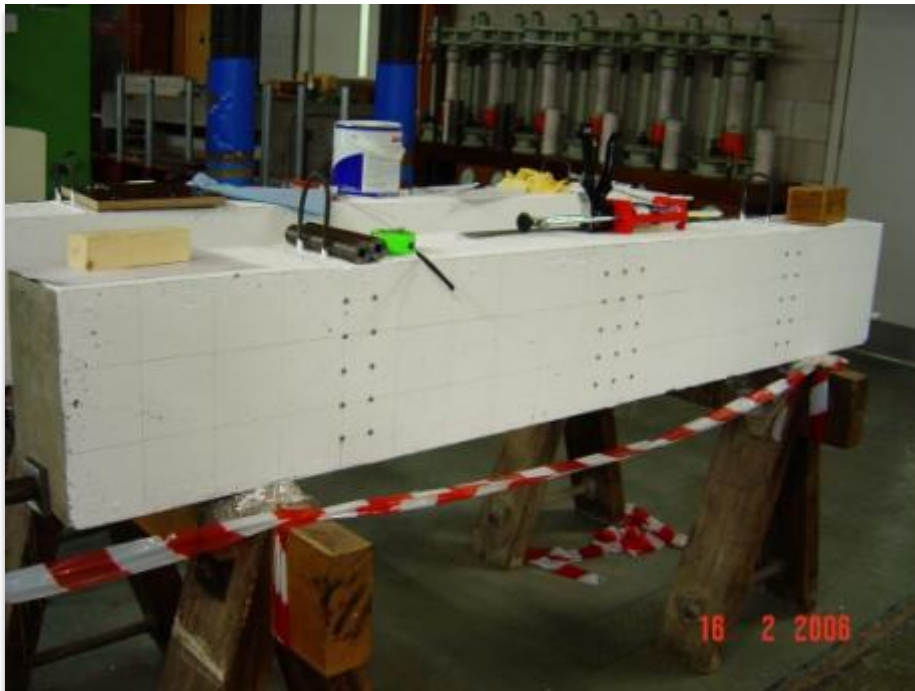
Figure 4.11: Demec studs glued in positions
