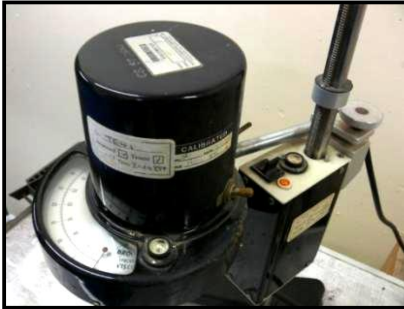
Figure 5.3: Brookfield Viscometer dial reading display
