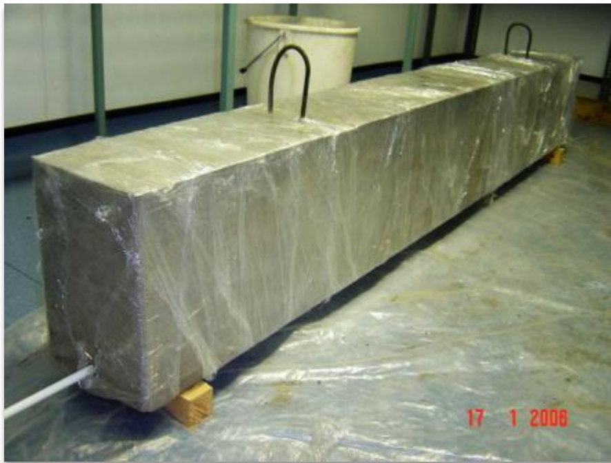
Figure 4.9: Beam wrapped in 'cling' film after formwork removal
