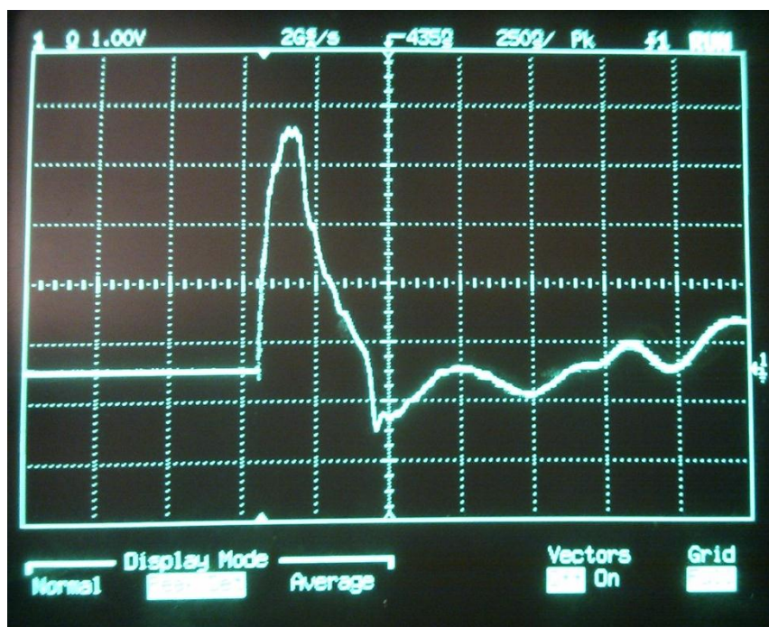
Figure 22. Showing a pulse from one of the 'successful' driver designs.
