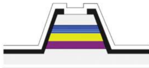
Figure 9. Example of a multi-cascade QCL with each cascade emitting at a different central wavelength. Such a system can provide a quasi-continuum over which to tune (8).
