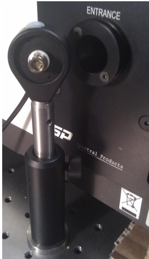
Figure 33. Improved PbSe Photodiode system, here the diode is mounted in a lens holder and can be positioned in the exact position where the laser beam should enter the monochromator. Alignment can then take place to maximise photodiode response before removing the photodiode and allowing the aligned laser light to enter the monochromator.
