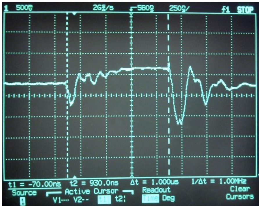
Figure 20. Example of one of the first pulses showing a perturbation of a dc source rather than a true pulse.
