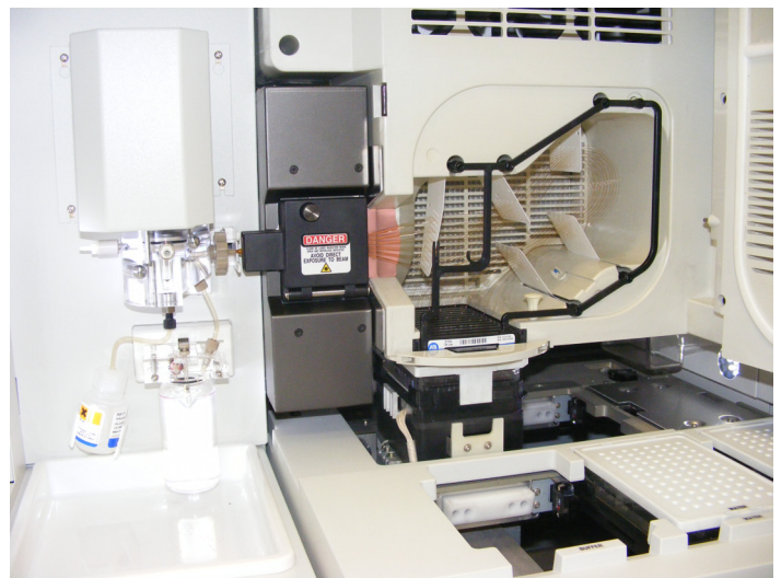
3730 DNA Analyser equipped with 48-capillary
