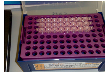
8-strip PCR tube with improvised holder
