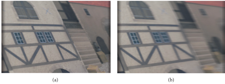
FIGURE 5: (a) is the refocus result by using the correct inclined plane parameters, and it is an all-in-focus image. (b) is the result by using wrong parameters, and it is noticed that there is only defocus blur in horizontal direction.
