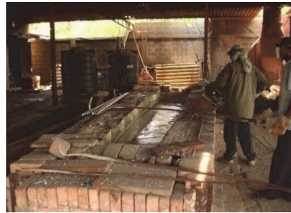
(b) Hot dipped @ 450° by immersion
