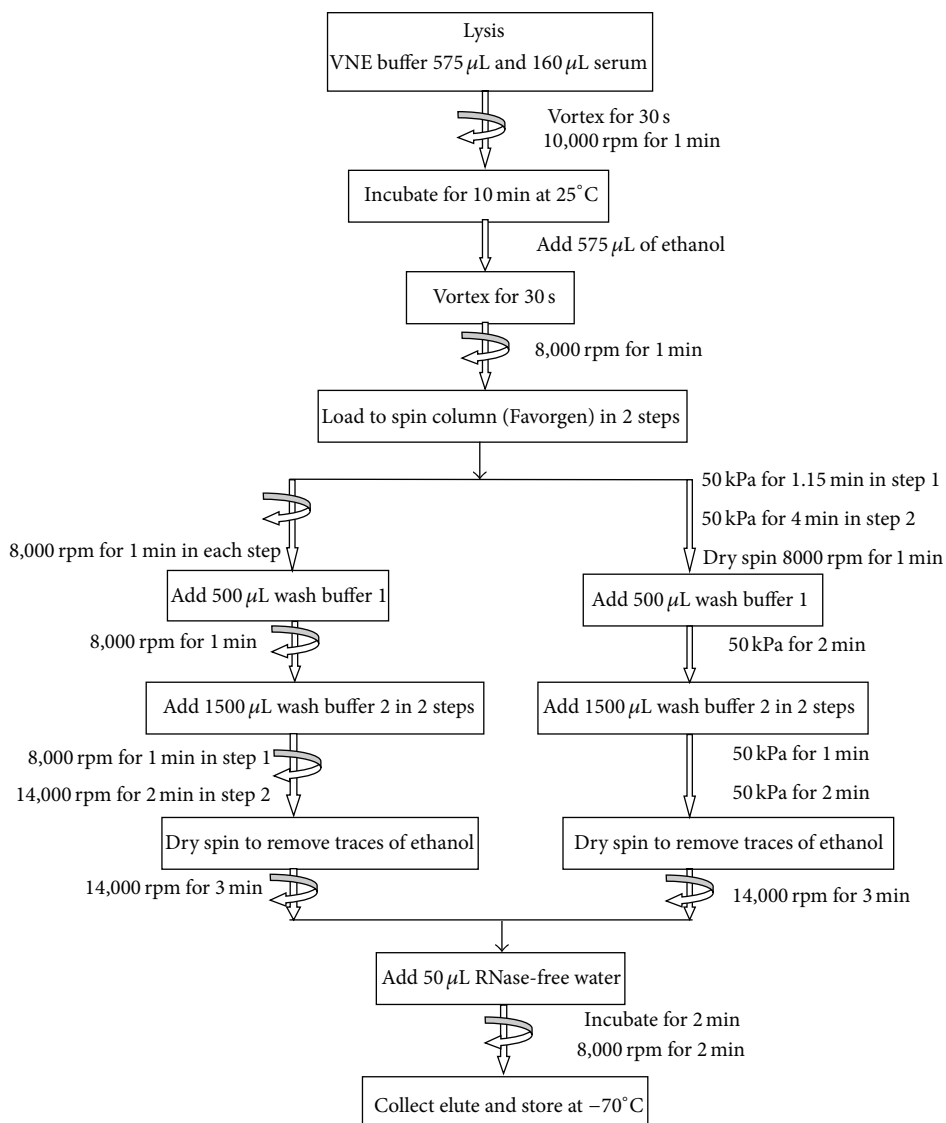
FIGURE 1: Spin and vacuum filtration based protocol for HCV-RNA extraction using Favorgen kit.
