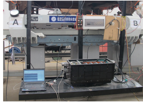
FIGURE 7: Full-scale single bogie of CMS-04 maglev train.
