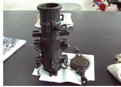
FIGURE 2: Soil compaction mould assembly modified from concrete specimen mould.
