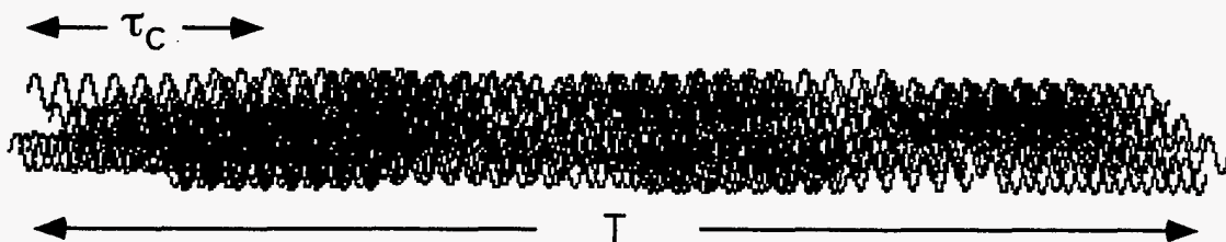
FIGURE 1. An example of chaotic light given by a random superposition of 100 sinusoidal wave packets each with six periods long. The total length of the pulse is T .
