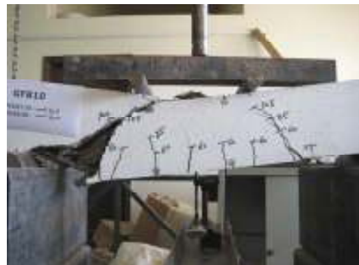
Figure 19 mode of failure GFB10
