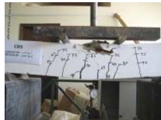
Figure 11 mode of failure CB5
