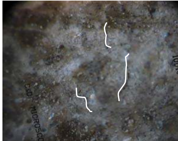
Figure 6 Shrinkage cracking on cigarette filter concrete
