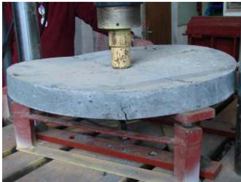
Figure 2 Round disc test setup
