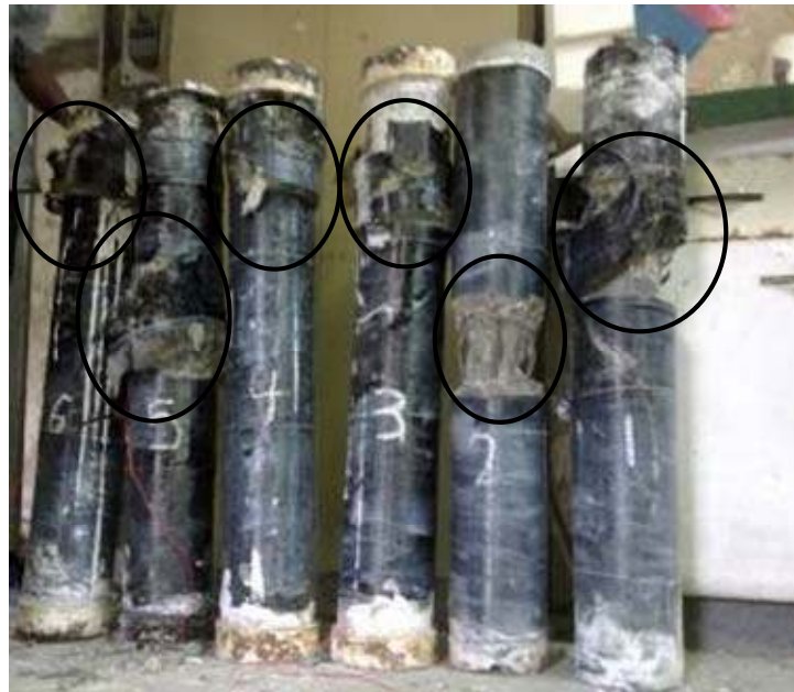
Figure 6 Failure modes for all columns
