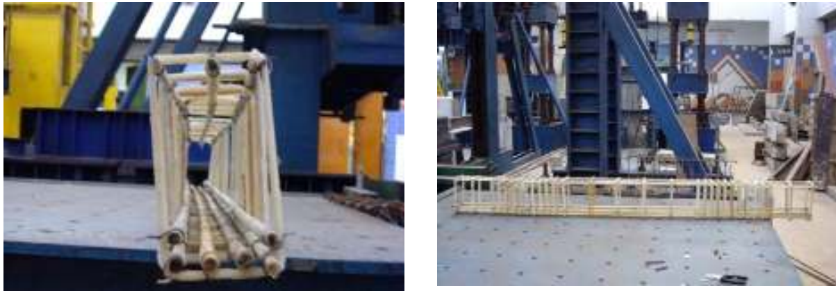
Figure 1 General view of GFRP bars and stirrups.
