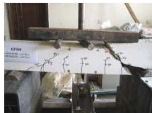
Figure 13 mode of failure GFB9
