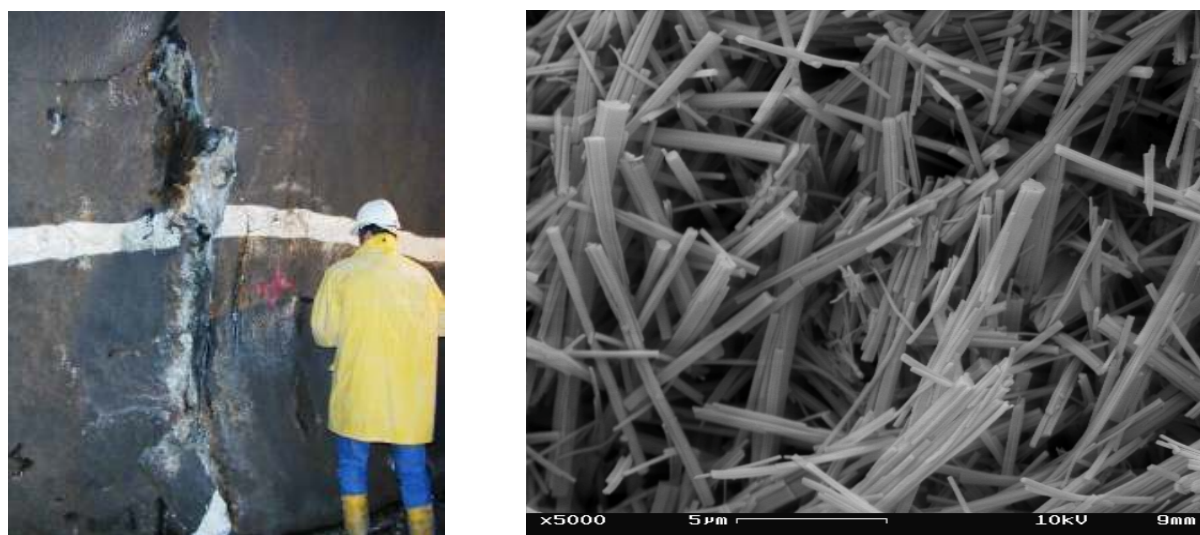
Figure 1 Concrete destroyed by thaumasite formation (left) and secondary electron image (SEI) of thaumasite crystals in deteriorated concrete (right)
