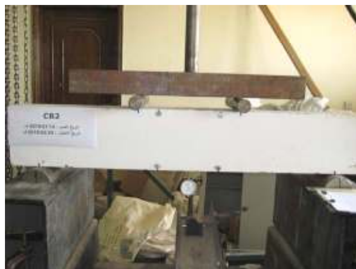
Figure 3 Model of the concrete beams load test
