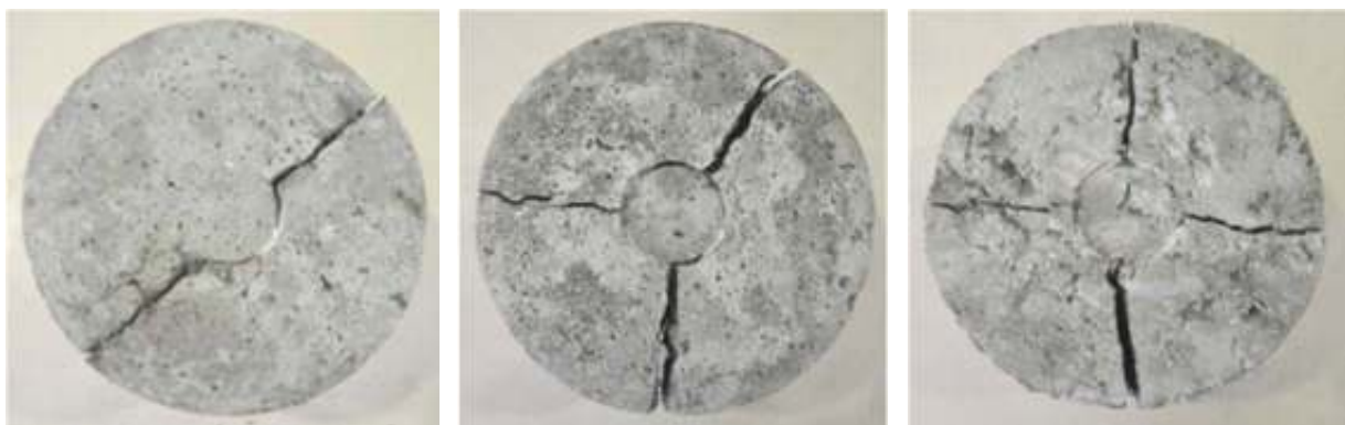
Figure 3 Final specimens state with typical cracks patterns
