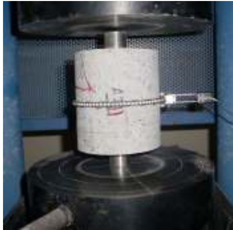
Figure 2 BCN test set up used
