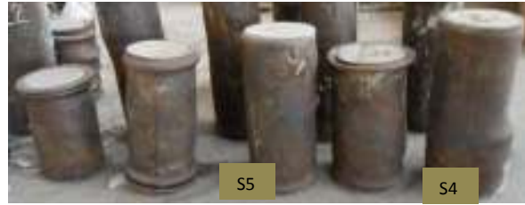
Figure 4 Buckling of the tube wall
