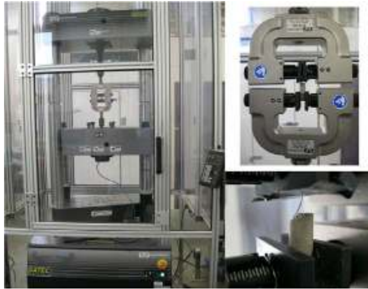
Figure 2 Instrument and specimen configuration for the single-fibre pullout test
