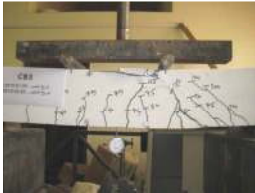
Figure 10 mode of failure CB3
