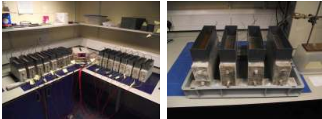
Figure 1 experimental setup for determination of corrosion rates
