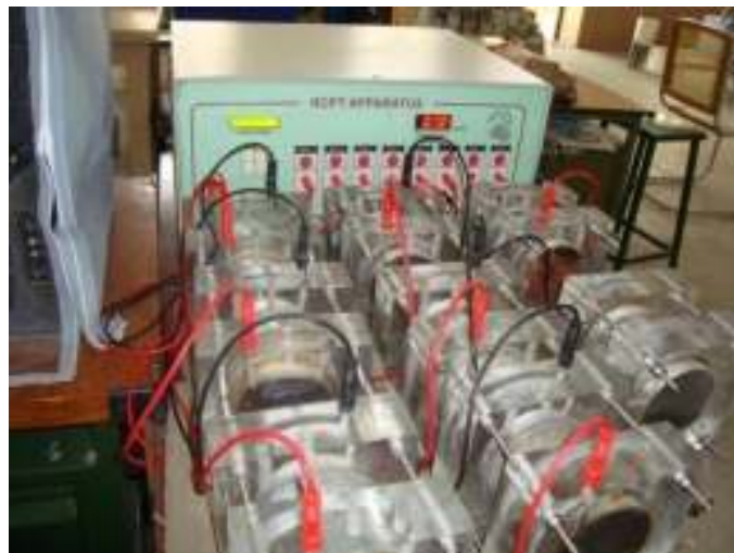
Figure 1 Multi-cell RCPT Apparatus with specimens
