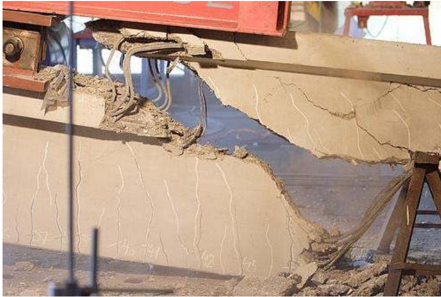
Figure 4 Breaking of beam F.P.02
