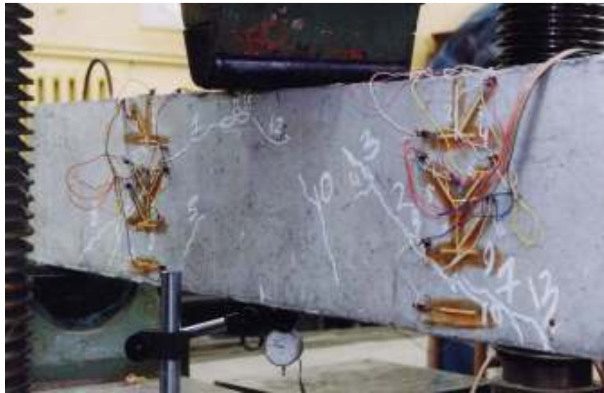
Figure 3 A three-point bending of concrete beam specimen
