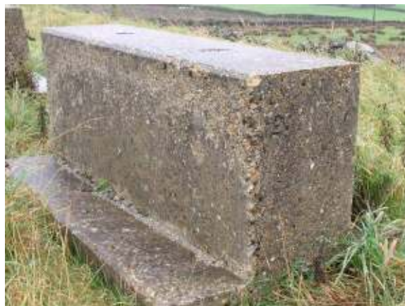
Figure 2 Non air-entrained 30 MPa Portland cement concrete exposed for 12 years and around 1100 freeze thaw cycles as measured by air temperature
