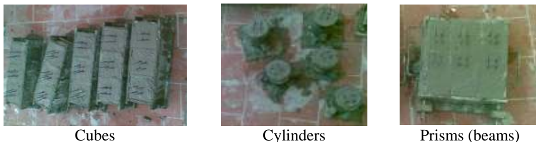
Figure 2 The specimens after casting and installing probes
