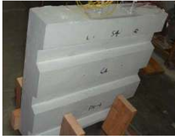
Figure 2 Typical type B shrinkage profile specimen
