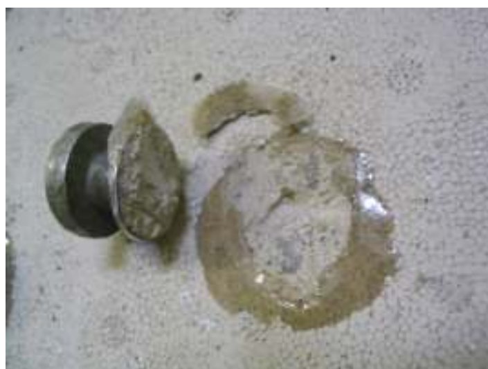
Figure 4 Cohesive failure of a joint (Pull-off test)
