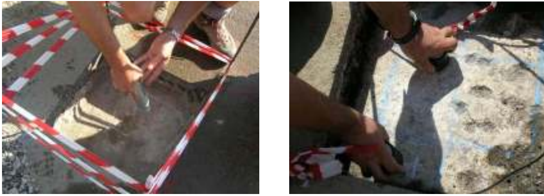
Figure 2 a) Schmidt rebound hammer test, b) Ultrasonic pulse velocity test on bridge slab
