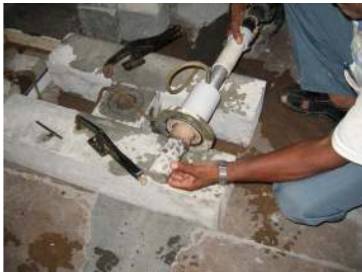
Figure 2 Core taken from the cube
