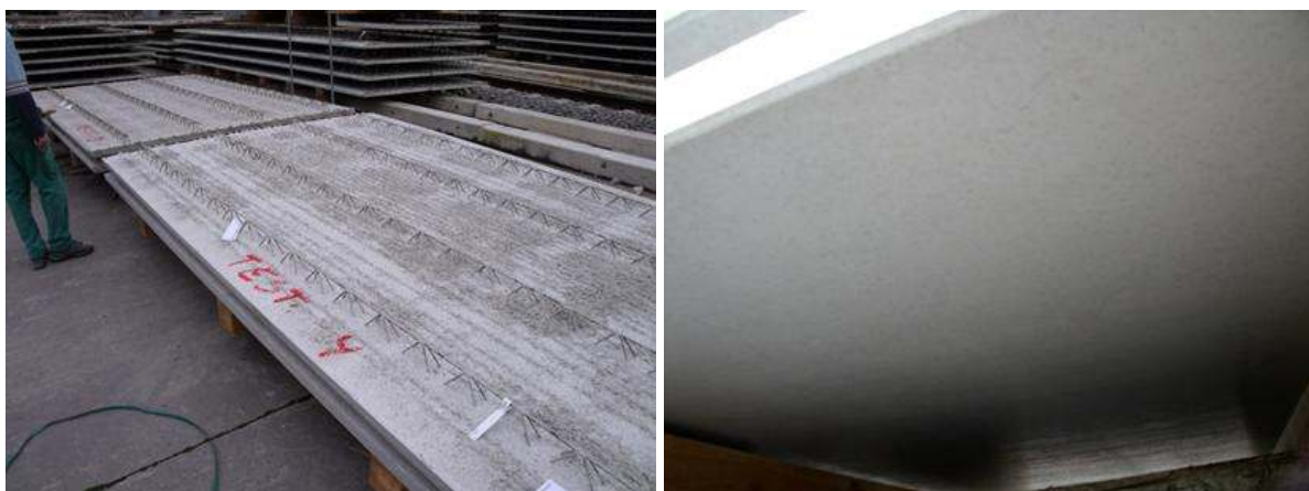
Figure 9 Fabrication of semi-finished slabs with cement reduced ECO-Concrete1 (left), finished surface, view from the bottom (right)
