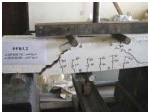
Figure 20 mode of failure PFB12
