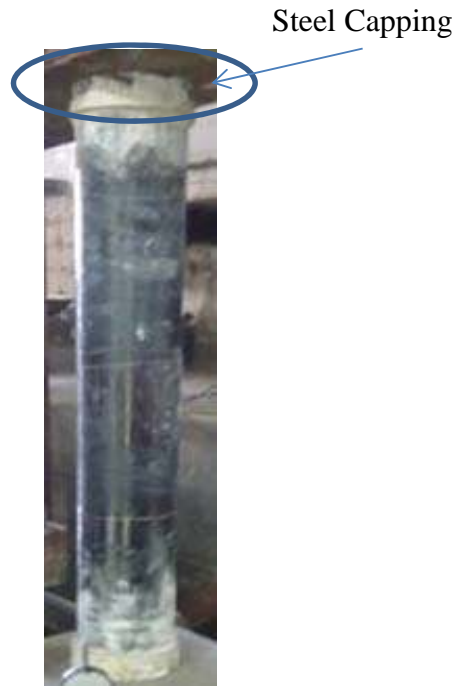
Figure 2 Confined column with steel capping before loading
