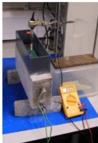
Figure 2 half-cell measurements for corrosion initiation
