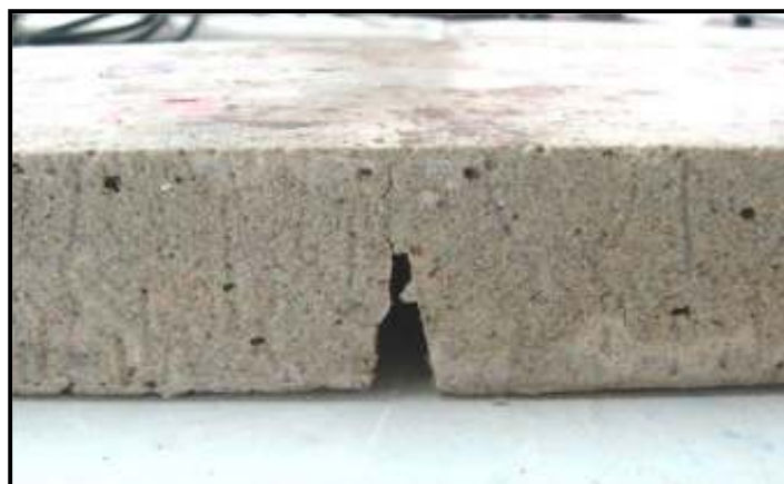
Figure 22 Typical appearance of specimen after prolonged number of wheel passes
