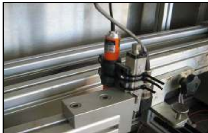
Figure 7 Additional TML LVDT for tests
