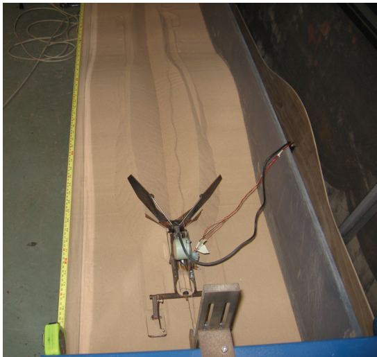
Fig. 8. Digital image of spoil heaps after test ( L = 1000 mm, h/L = 0.1 )
