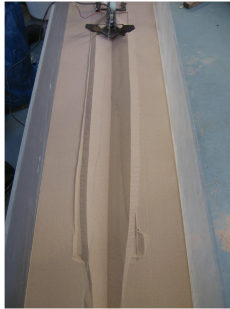
Fig. 4. Photograph taken at the conclusion of the flat bed plough test showing the ploughed trench and the spoil heaps.
