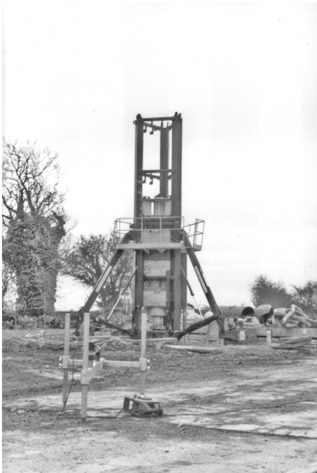
Fig. 1. 3 MN Statnamic testing device
