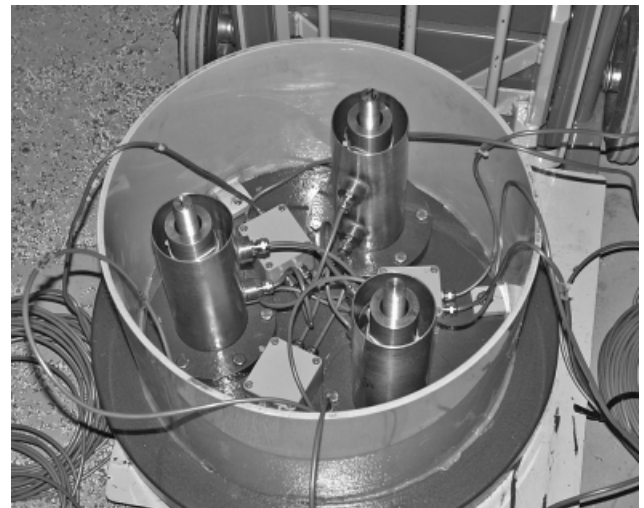
Fig. 5. Pile-tip load cell with top plate removed and load columns visible
