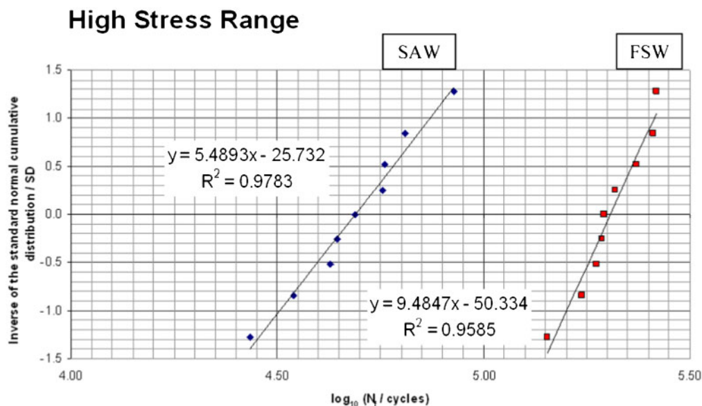
6 Comparison between SAW and FSW fatigue testing for all thickness of welds produced
