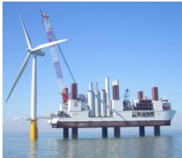
Figure 1: Example of a jack-up vessel being used for offshore wind turbine maintenance [4].
