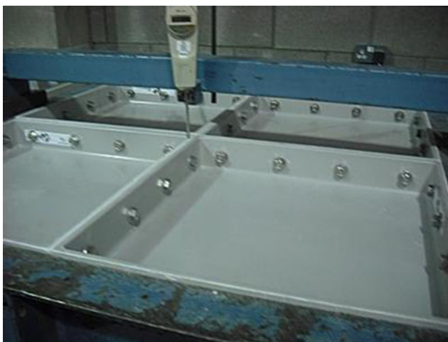
Fig. 2 Four panel bolted assembly bolted on to the rupture testing rig. The deflection meter is placed at the cruciform area
