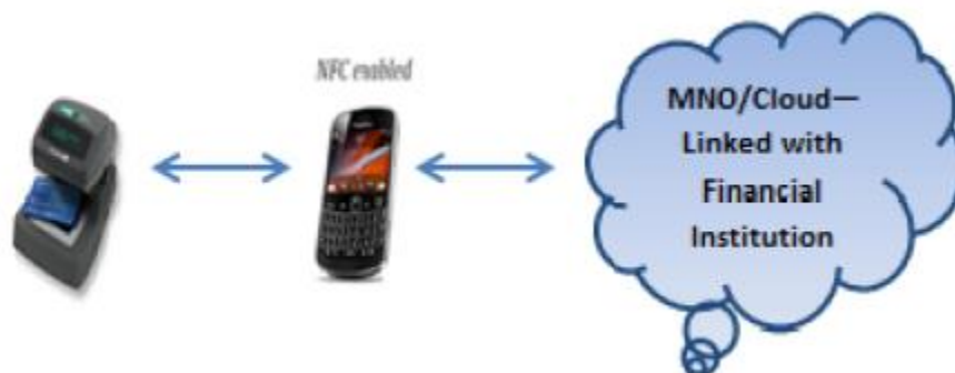
Figure 18: POS and MNO Communicating through NFC Phone
