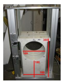
The aperture is 160 mm diameter and the vertical travel is 165 mm. Note that there are 3 locations marked around the aperture: MPA-A, MPA-B and MPA-C.
