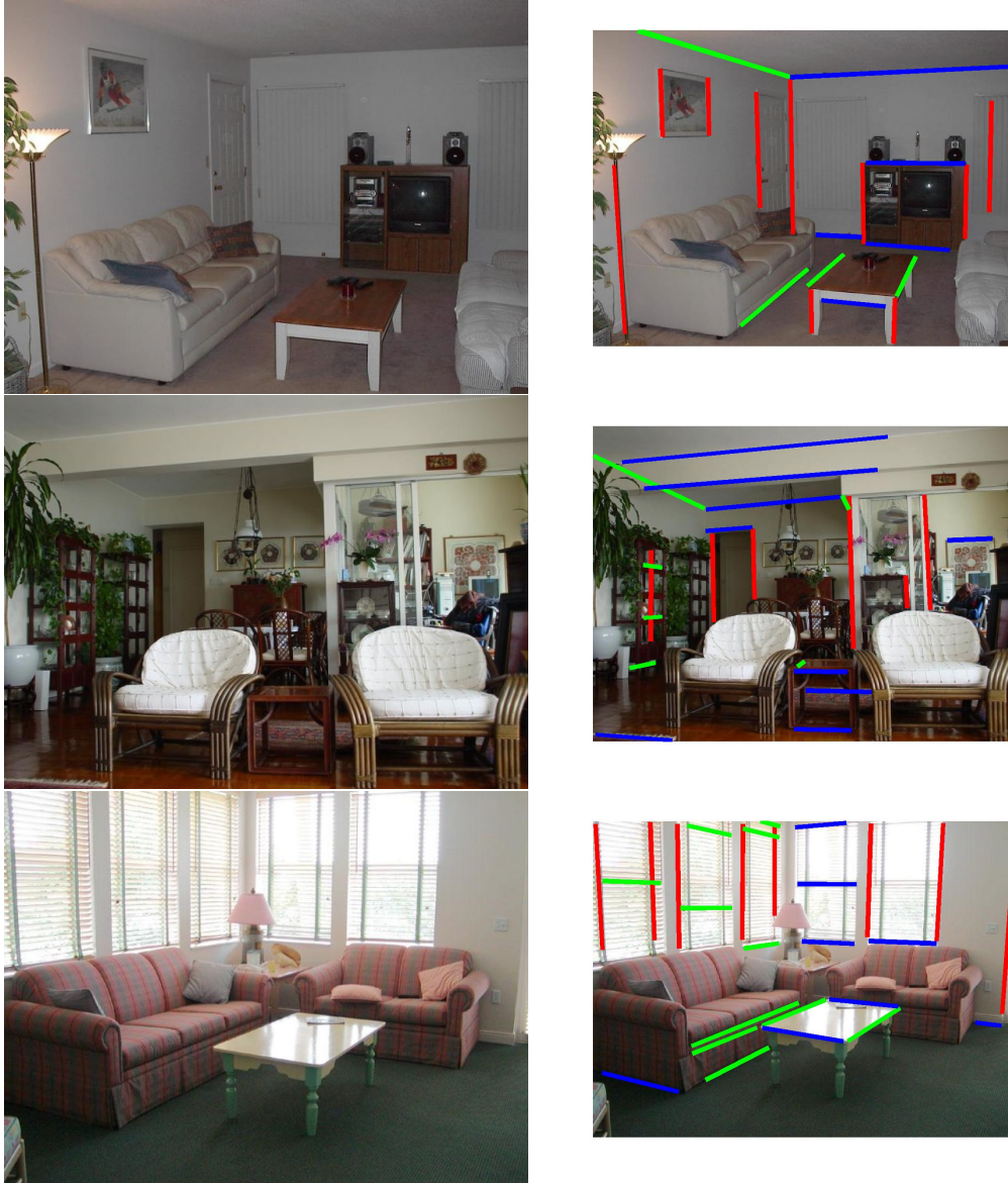
Figure 3.3: Examples of images shown along with the ground truth lines in each of the three orthogonal directions. These lines are then used to determine the vanishing points in each of these directions.
