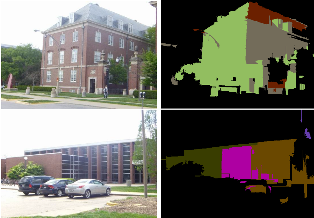
Figure 4.6: The left image shows the original image and the right images are these images with the vertical planes identified and clustered into individual planes
