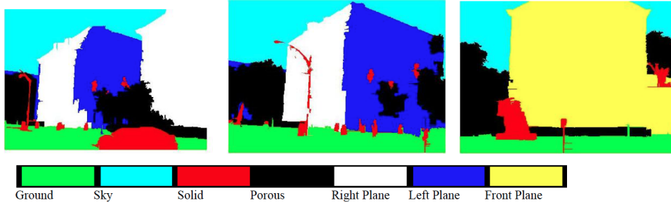
Figure 1.3: The top row shows images from the dataset overlaid with their ground truth labels, indicating which 3-D surface each pixel belongs to. An index for these labellings is beneath the images.
