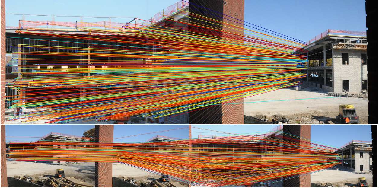
Figure 2: (Top) FANN matcher returns 685 matchings. Although it is robust to viewpoint change, some bad matches such as the lower-right keypoint of the right image still persist. (Bottom) Tracker groups similar matched keypoints across four images. Bad matches are further filtered.
