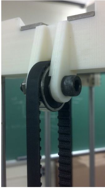
Figure 5.8: Closeup of the “top corner.” A radial bearing is used as an idler bearing for the timing belt. By tightening the M8 bolt, the 3D printed part clamps on the idler’s inner race.
