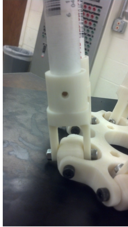
(b) U-joints used in “ankle” joints
