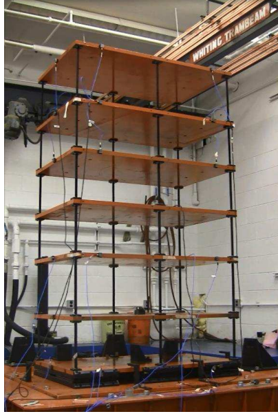
Figure 8.1: Photograph of the six-story base-isolated building model
