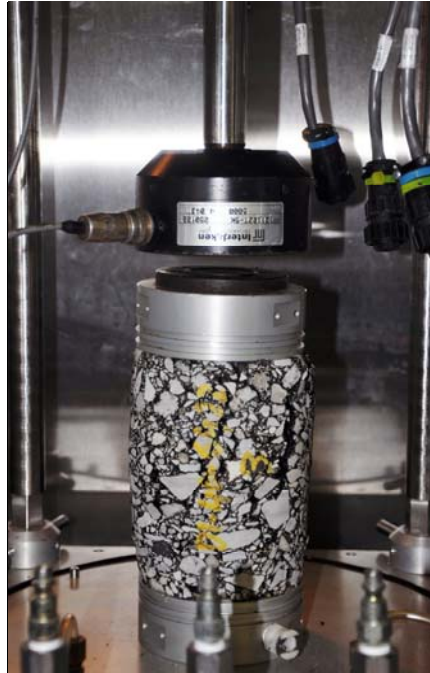
Figure 4.3. A specimen at the conclusion of a flow number test.
