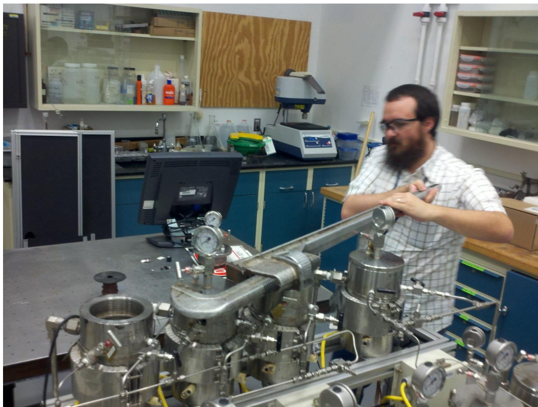
Figure 54. Static reactor vessel holds pressure and temperature conditions for the experiment (2000 psi at 50°C).
