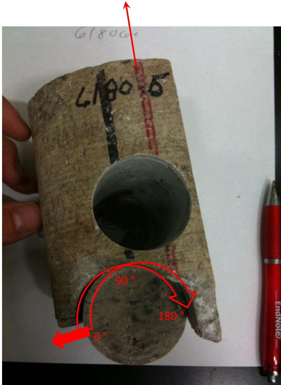
Figure 12. The measured core is normal to bedding. The line at the top indicates the upwell direction. The curve describes the rotation of the core along which velocities were measured.
