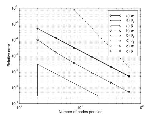
Figure 3: Bending solutions for a thin-plate problem. Load cases a, b, c and d. Relative error for the unknown fields w,  $\theta_2$  and  $\beta$  versus number of nodes per side. The attainment of the  $h^2$  convergence rate in the  $L^2$  error norm clearly appears.
