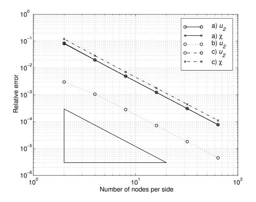
Figure 1: Membranal solutions for a thin-plate problem. Load cases a, b and c. Relative error for the unknown fields  $u_2$  and  $\chi$  versus number of nodes per side. The attainment of the  $h^2$  convergence rate in the  $L^2$  error norm clearly appears.
