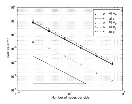
Figure 2: Membranal solutions for a thick-plate problem. Load cases a, b and c. Relative error for the unknown fields  $u_2$  and  $\chi$  versus number of nodes per side. The attainment of the  $h^2$  convergence rate in the  $L^2$  error norm clearly appears.
