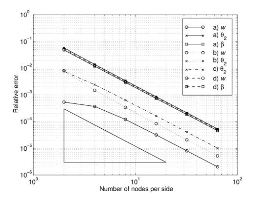
Figure 4: Bending solutions for a thick-plate problem. Load cases a,b,c and d. Relative error for the unknown fields w,  $\theta_2$  and  $\beta$  versus number of nodes per side. The attainment of the  $h^2$  convergence rate in the  $L^2$  error norm clearly appears.
