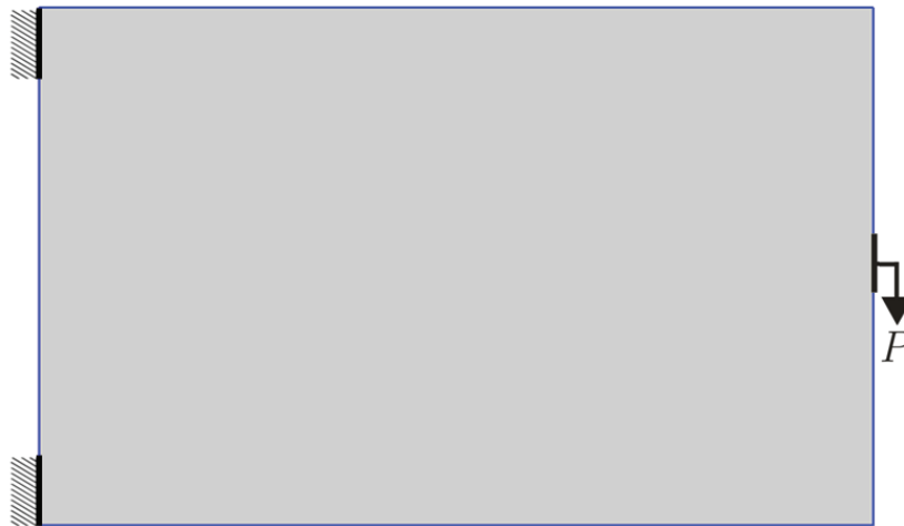
Figure 7.12: Design domain, loading and boundary conditions for cantilever beam.
