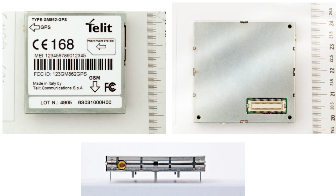
Figure 5.4: The Telit GM862-GPS
