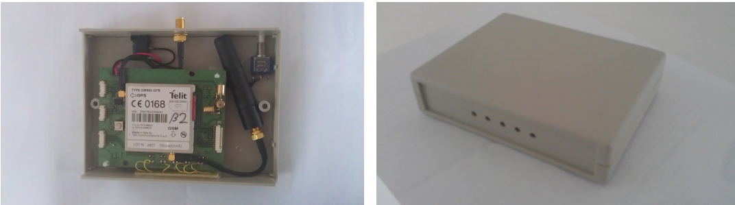
Figure 5.9: Tracker (v.3.1), in the 2nd box design
