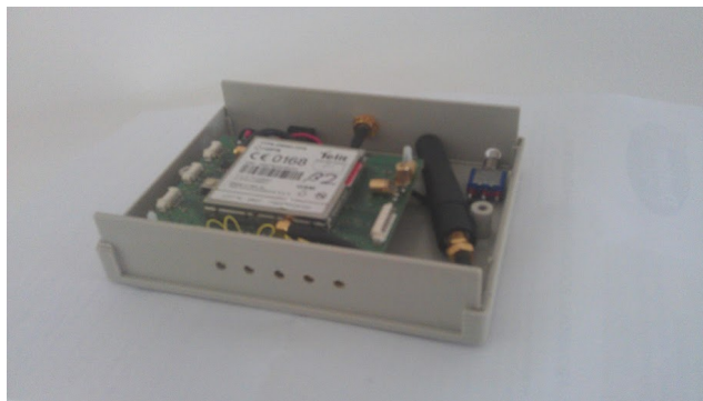
Figure 5.2: A v.3.2 Durham Tracker, showing the current state of the project
