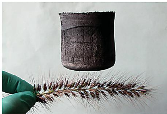
Figure 1.04: A cylinder of carbon aerogel (volume ca. 100 \text{ cm}^3 ) is sufficiently lightweight that it does not deform fine plant fibres. Image reproduced from reference 29.
