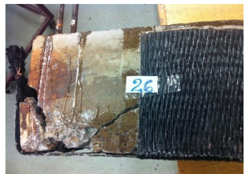
Fig. 12 Photographs of failed beams
