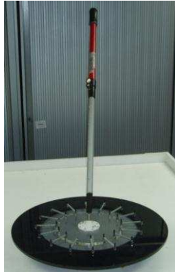
Figure 3, Hand held stick on a disc with omni-directional wheels
