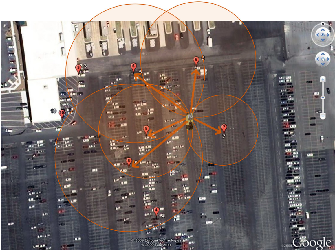
Figure 95: The multilateration localization technique as conducted in a real-world large parking lot environment that is RF covered by a wireless sensor network. Identical unique identification packets are broadcasted by the NF-CoA wireless connectivity module and captured by multiple fixed anchor nodes for multilateration purposes.
