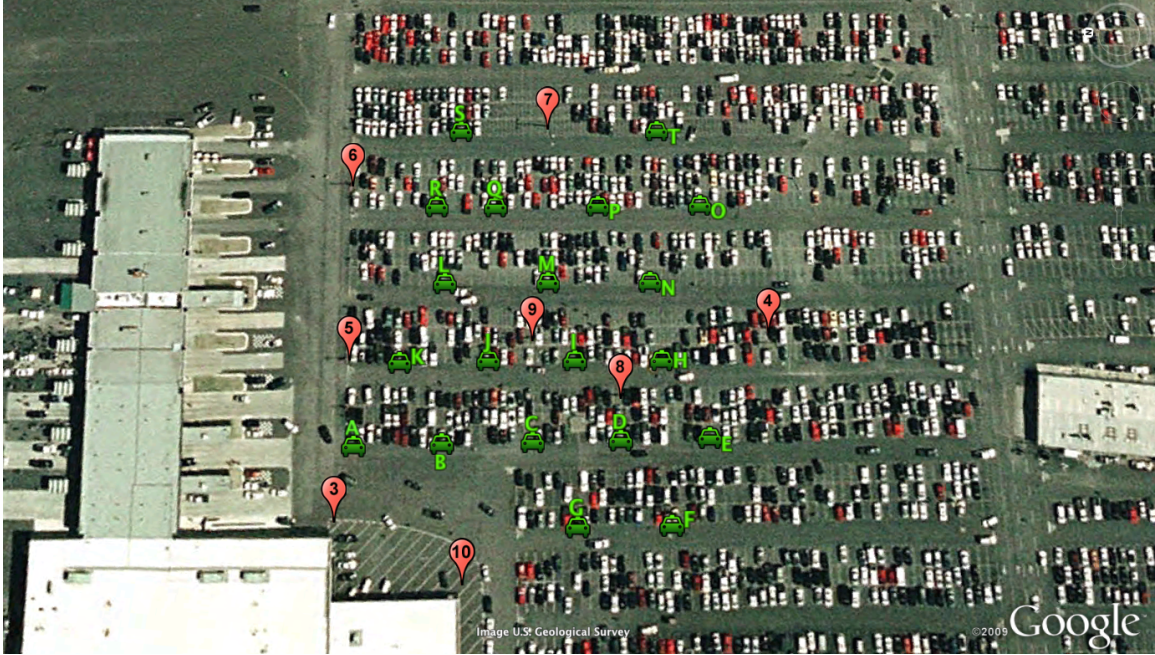
Figure 97: The WSN topology and measurement positions within a large parking lot.
