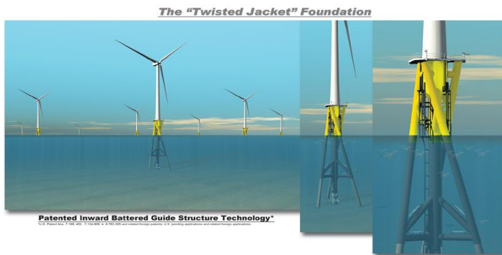
Figure 7: Twisted Jacket foundation, supported by the UK CT OWA. A prototype was installed to support the meteorological mast at the Hornsea future offshore wind farm. Drawing courtesy Keystone Engineering
