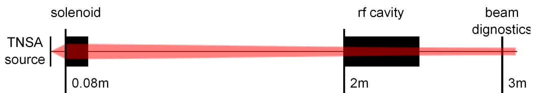
Figure 4.4: The 150 mm long pulsed solenoid is positioned 80 mm behind the laser target (40 mm from target to the stainless steel vessel surrounding the solenoid) and is typically set to focus 9.6 MeV protons at 3 m. The cavity (550 mm long) starts at 2 m and is followed by a diagnostic box at 3 m, where RCF stacks, the diamond ToF detector and a compact magnetic dipole spectrometer can be placed.
