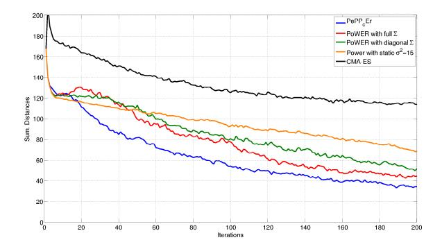
**Figure 4.3.:** Comparison between PePP<sub>c</sub>Er , PoWER and CMA-ES on the inverse kinematic task with a 26-linked robot arm. In each iteration we generated 50 parameterized joint configurations and used the 25 best samples. Every Algorithm was performed with 30 trials and plotted with his mean.
