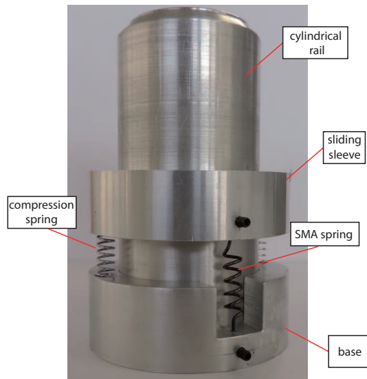
Figure 9.11: Sliding sleeve dummy system
