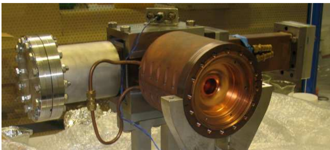
Figure 5.1. The VELA/ALPHA-X photoinjector gun.
