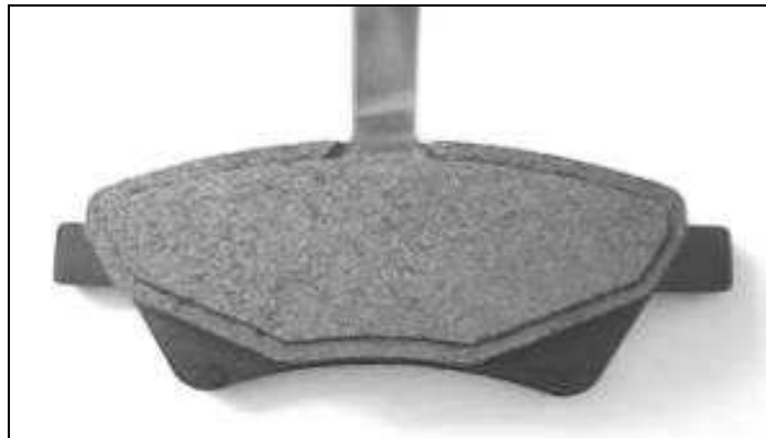
Figure A.3 Pad assembly with film laminate sandwiched within pad
